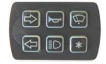
This image is the actual size of the 6-Button HC Keypad. L48mm W30mm D13mm (incl. buttons)
