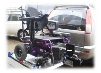
Swing-Away option allows an unoccupied outside lift to be easily pivoted away from the vehicle
